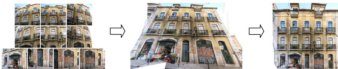
Figure 1 – Stitching and perspective correction processes used to obtain an elevation type of façade image.
