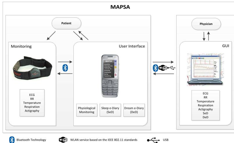
Figure 1: MAPSA system architecture.
