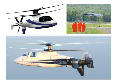
Figure 1.2: The Sikorsky's X2 Technology Demonstrator. Top Left: concept model. Top Right: flight testing in August 2008. Bottom: flight testing in September 2010. (*Courtesy of Sikorsky Aircraft Corp.*)
