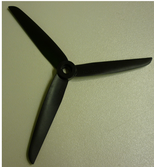
Figure 4.6: GWS 7x3.5x3 nylon propeller (left handed).
