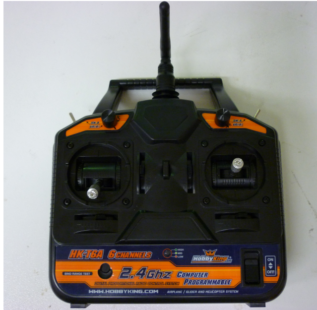
Figure 4.13: HKT6Av1 radio transmitter.
