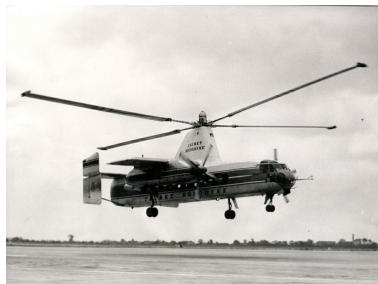
Figure 2.5: The Fairey Rotodyne, a compound helicopter with VTOL capability.
