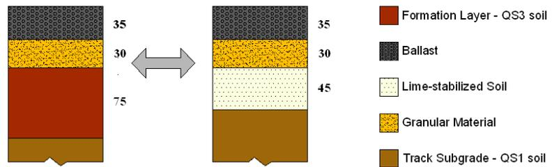
**Fig. 7 Definition of sections obtained for clay subgrades**
