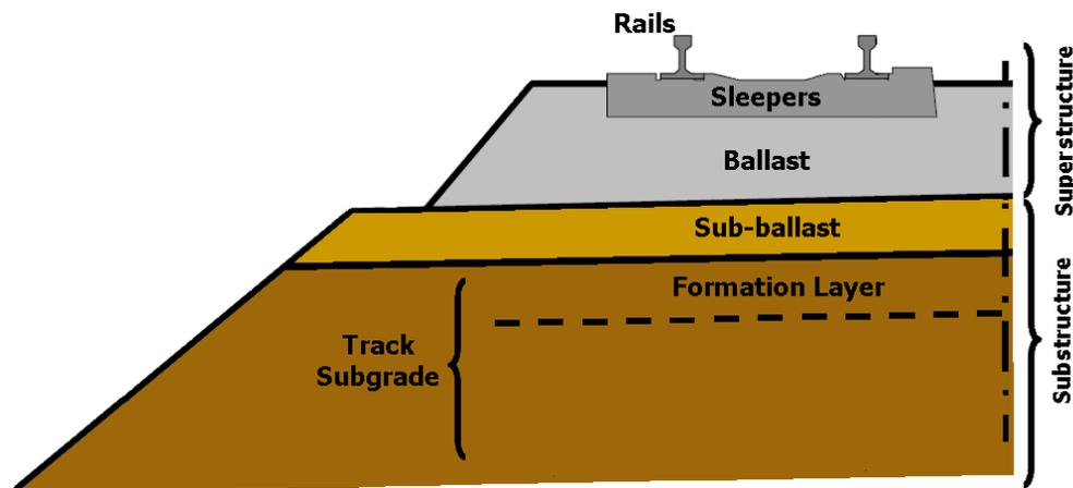
**Fig. 1 – Elements of a railway – Super and substructure**
