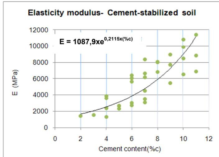
Fig. 3 – Elasticity modulus versus Cement content
