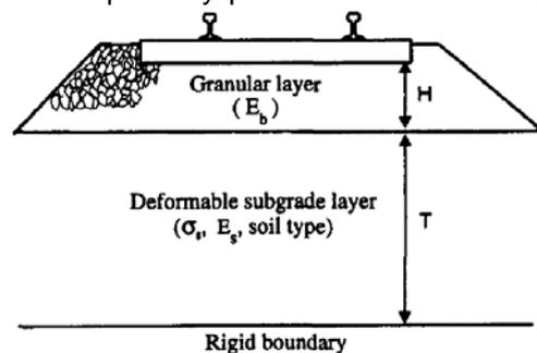
**Fig. 4 – Design of clay track subgrade. Li and Selig [10]**
