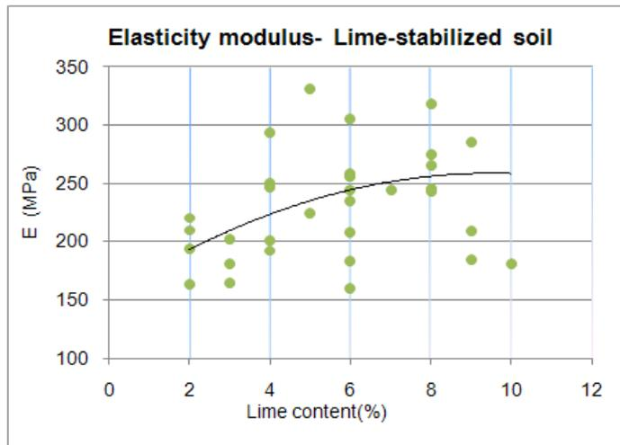
**Fig. 2 – Elasticity modulus versus Lime content**
