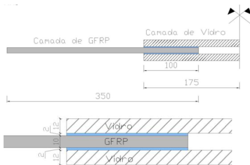
Figure 12 – Geometry of the specimens used on double lap joint tests: section view (top) and detail of the overlap zone (bottom).
