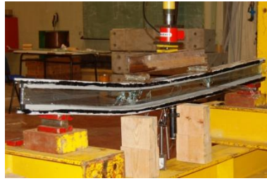
Figure 21 – Beam I-PU: deformation and overview of crack propagation before unloading.
