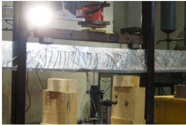
Figure 20 – Beam R-PU: crack propagation before ultimate failure.
