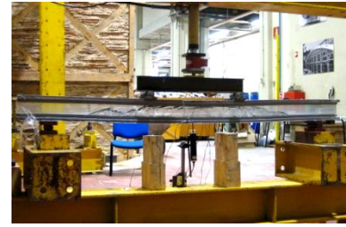
Figure 22 – Beam I-EP: crack propagation before ultimate failure.
