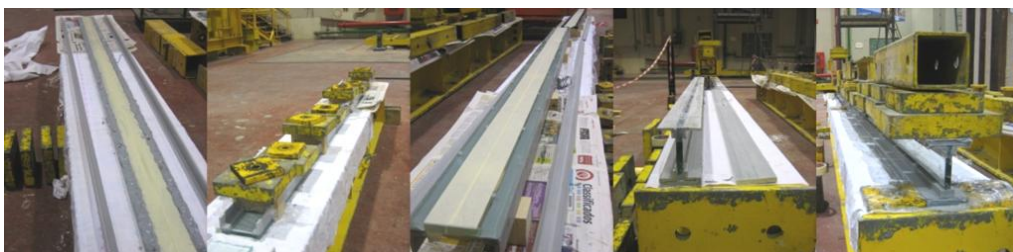
Figure 17 – Different stages of I section composite beams fabrication process.
