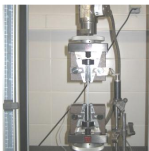
Figure 9 – Tensile tests in structural adhesives.
