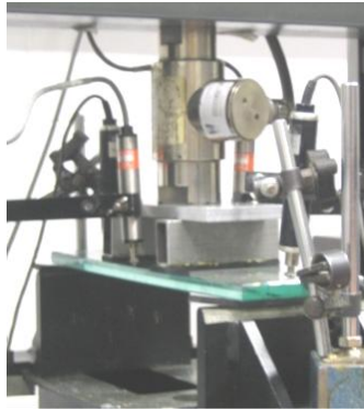
Figure 7 – Flexural tests in annealed glass panes.
