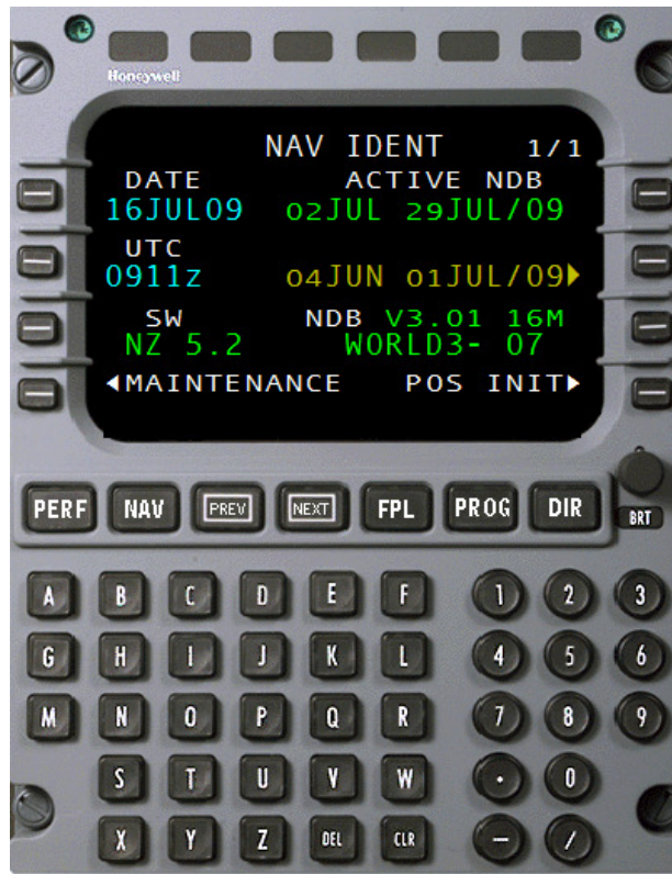
Figure 4-2 - Embraer ERJ145 Honeywell FMS CDU
