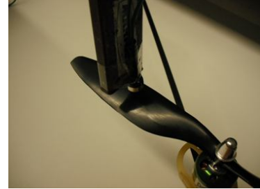
Fig. 5. Microphone positioned to record the propeller sound.
