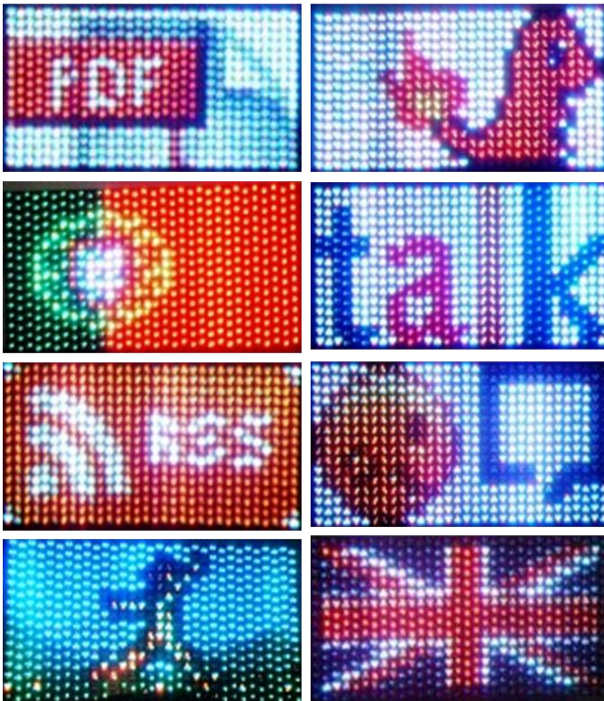
Fig. 11 Examples of 32x16 images on the display.
