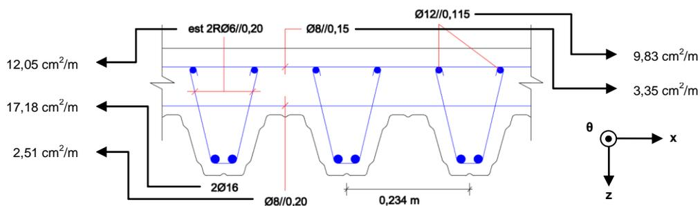
**Fig. 5.2 – Rebar adopted in the Weather Shelter – distribution and quantities per meter.**
