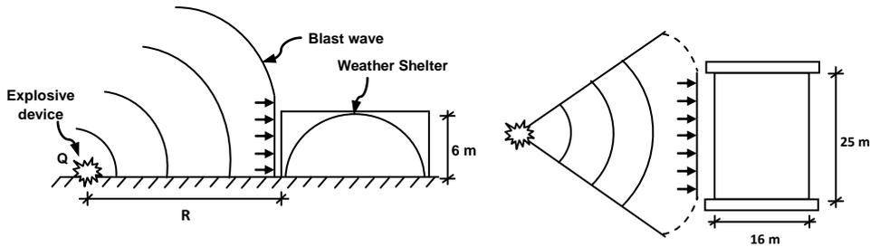
Fig. 6.2 – Blast wave representation on the Weather Shelter: side view (in the left); top view (in the right).
