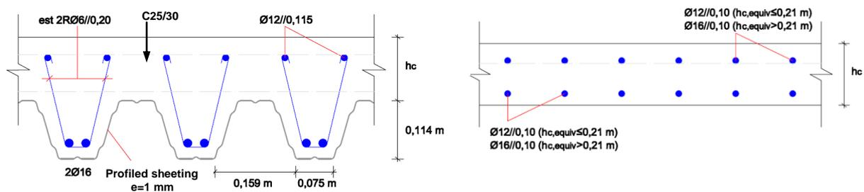
Fig. 6.1 – Transverse section considered for strength evaluation:  $\theta$  direction (in the left);  $x$  direction (in the right).
