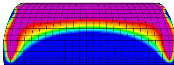
**Fig. 5.3 – Longitudinal stress on the top face of the shell.**
