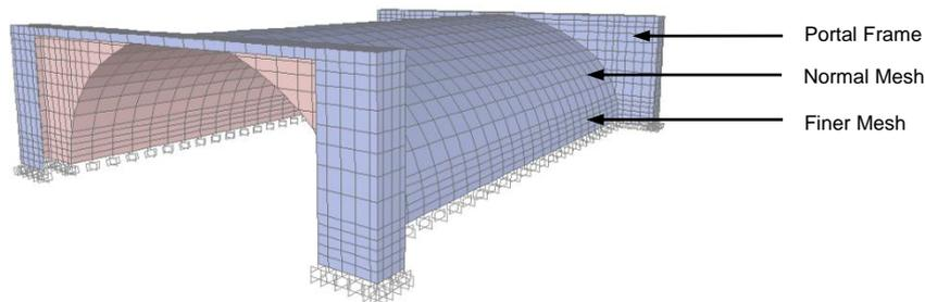
**Fig. 5.1 – Weather Shelter’s finite element model in SAP2000™ software.**
