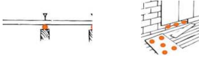
Figure 17 - Floor and Panel Fixing
