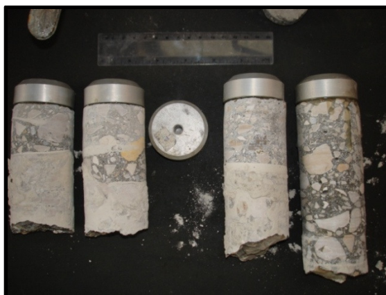
Image 10 – Illustration of the different types of rupture of the cores from the pull off tests
