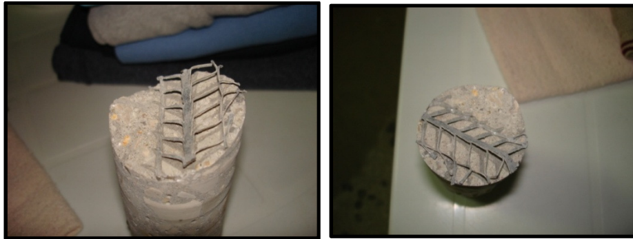
Image 13 – Raised ribs from the expanded metal mesh
