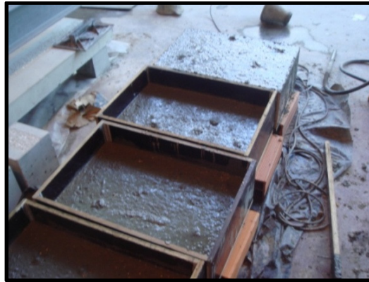
Image 6 – Concrete pieces of group I at the end of the first concrete pour. At the bottom of the image a monolithic piece from group 0.
