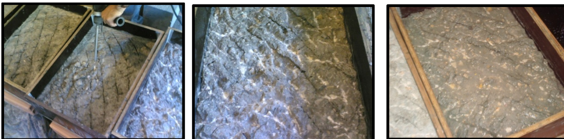
Image 9 - Aspect of the joint substrate surface obtained by the chipping of the substrate
