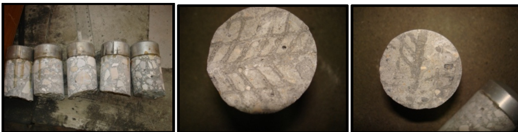
Image 14 – Roughened surface obtained by the expanded metal mesh
