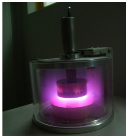
Figure 2.10 - Gold deposition by sputter coating to make the surface of the master mold electrically conductive.
