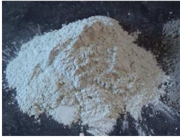
Fig. 1: Waste generated in the cutting process of GFRP (GFRPW)
