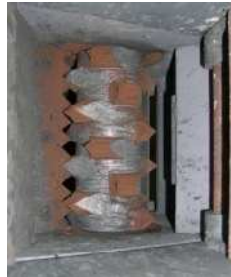
Fig. 2: ERWICH grinder's rotor: cylindrical shape
