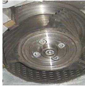
Fig. 3: RETSCH grinder's rotor: helical shape
