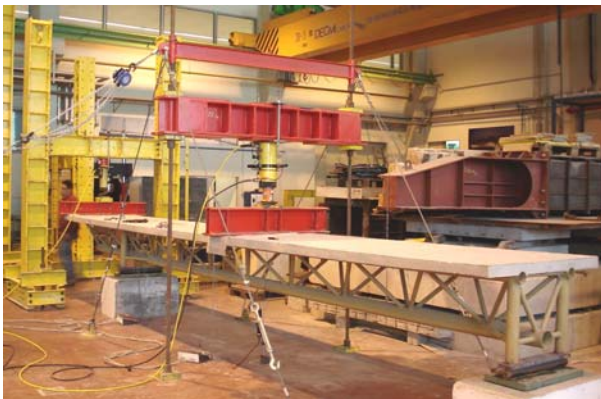
Fig. 7 - Test set-up and loading fixture.
