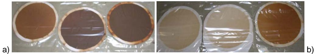
Figure 18 – Different coloration of the filters after the tests: a) MAG; b) CMT
