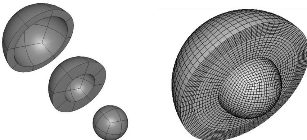
**Figure 1.** Computational model of the three parts and consequent discretization in finite elements.
