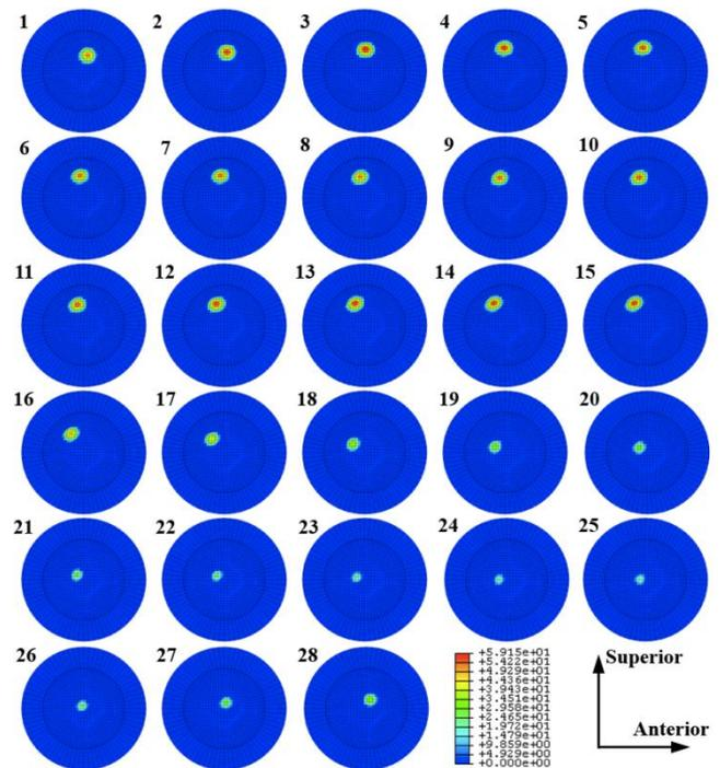
**Figure 7.** Contact pressure on the 32 mm model for the 28 instances of the gait cycle (CoCr – CoCr).
