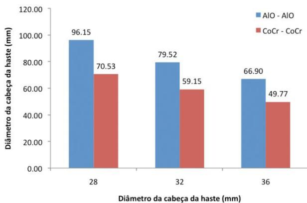
**Figure 10.** Contact pressure on the on the instance 4 for the different diameters.
