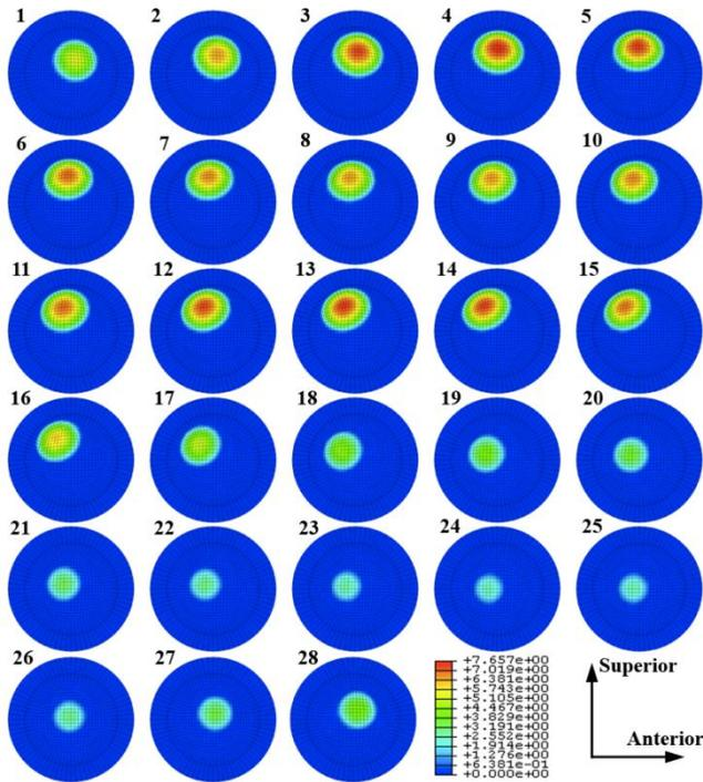
**Figure 5.** Contact pressure on the 36 mm model for the 28 instances of the gait cycle (PE – CoCr).
