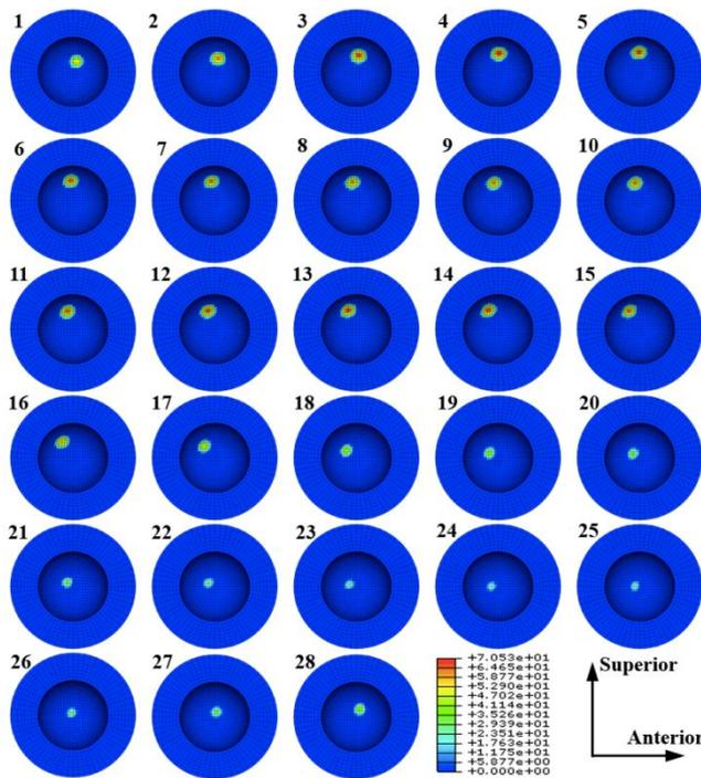
**Figure 6.** Contact pressure on the 28 mm model for the 28 instances of the gait cycle (CoCr – CoCr).
