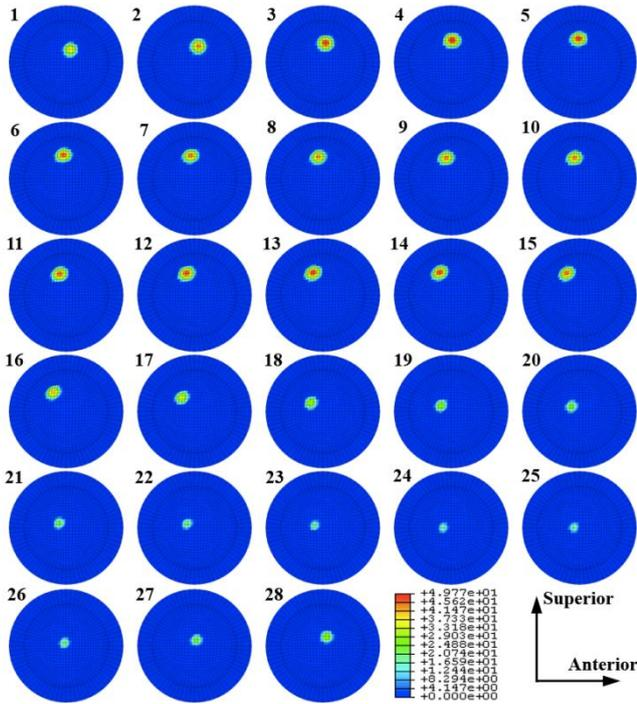
**Figure 8.** Contact pressure on the 36 mm model for the 28 instances of the gait cycle (CoCr – CoCr).
