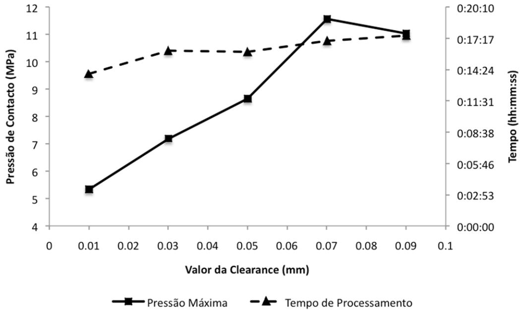
Figure 2. Influence of the clearance value on the contact pressure.
