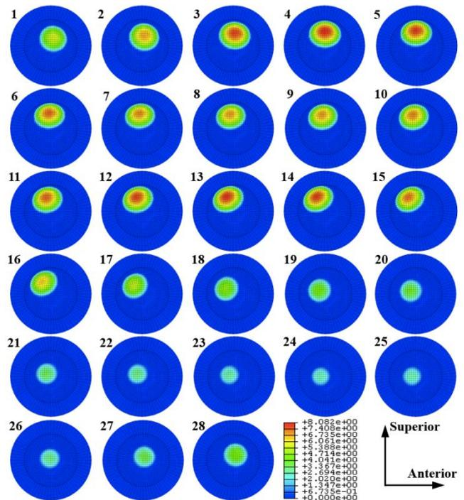
Figure 4. Contact pressure on the 32 mm model for the 28 instances of the gait cycle (PE – CoCr).
