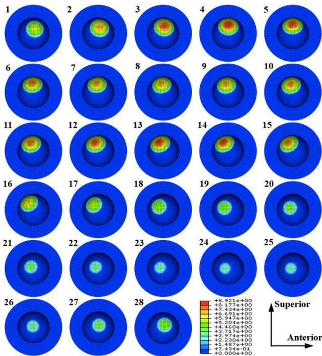
Figure 3. Contact pressure on the 28 mm model for the 28 instances of the gait cycle (CoCr – CoCr).
