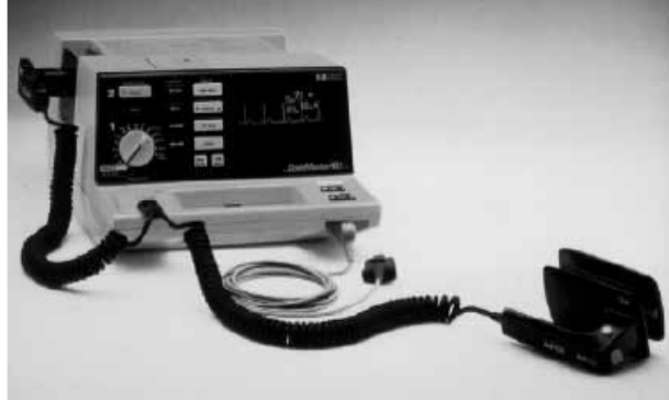
Figure 1.3 – Commercial pulse oximeter incorporating the emission and detection spring and the recording equipment [3].
