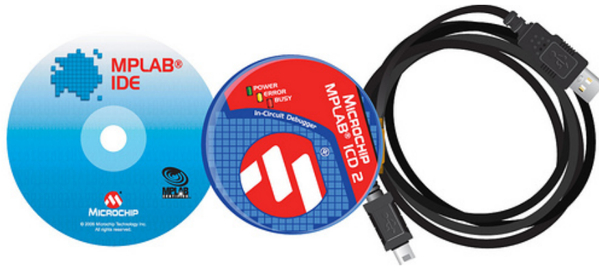
Figure 2.7 - Microchip® Development Kit: MPLAB® IDE development software and MPLAB® ICD2 interface between the PIC MCU and the computer [12].
