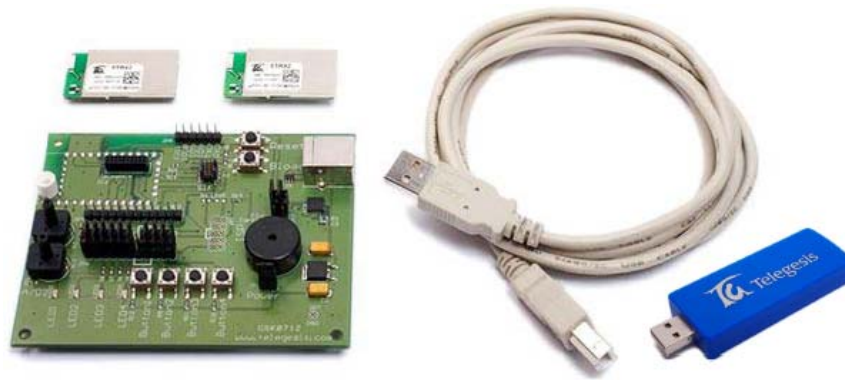
Figure 3.5 - Telegesis® Development Kit: development board, STRX2 transceivers and USB stick [25].
