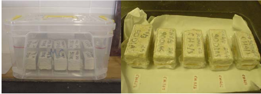
Fig. 2 – Salts crystallization – Procedure 1
