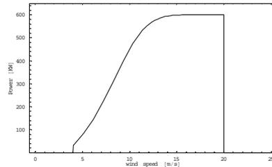
Fig. 7. Power curve of a Vesta V44 600/44, with nominal capacity of 600kW.
