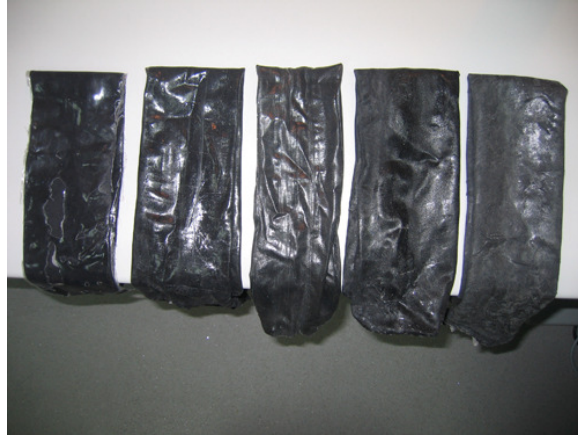
Figure 35 - Lycra fibre in silicone matrix composite material for the wing skin
