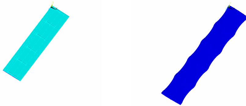
Figure 14 - wing model showing (above) the undeformed and stretched skin
