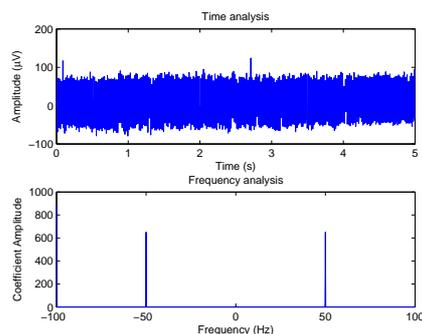
**Figure 18:** Designed DAQ signals preliminary analysis. Upper plot - 5 second signal. Lower plot - Frequency analysis of the acquired signal.
