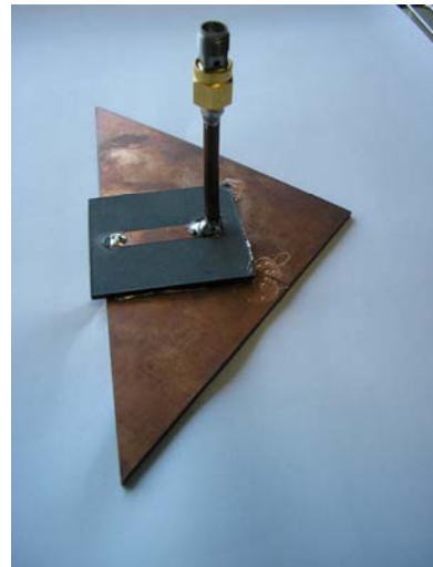
Fig. 11. Photograph of the back side of the prototype of the triangular antenna with ideal switches. In this image we can see the coaxial cable and the microstrip transmission line.
