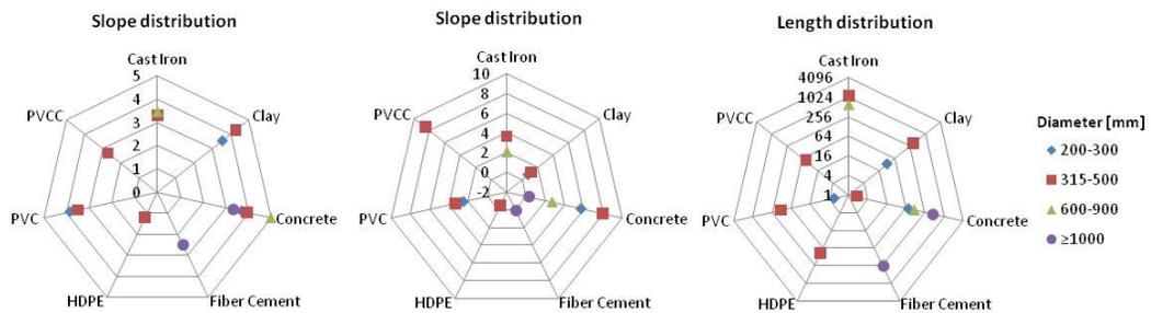
**Figure 1** – Depth, slope and length distribution of the sewer reaches of Chelas subsystem.
