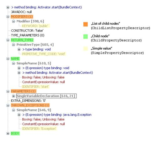
Figure 3.1: Structural properties of a Java method declaration
