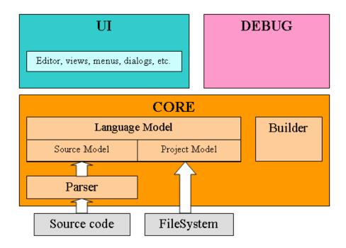
Figure 2.2: Basic IDE Architecture
