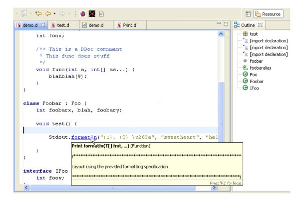
Figure 4.1: Text hovers and hyperlinking in the D IDE implementation
