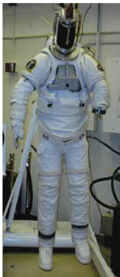
Figure 6 - Robot used to test spacesuits with the EMU (present spacesuit used on the space shuttle)
