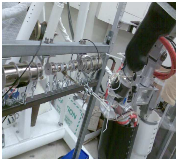
Figure 23 - Calibration of the torque of the arm joints
