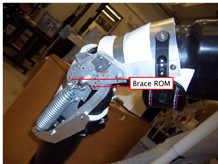
Figure 33 - View of two of the four screws used to change the limits of the range of motion.
