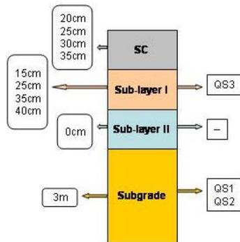
Fig. 6 – Combinations of material type and thickness for granular reinforced with cement sub-ballast.
