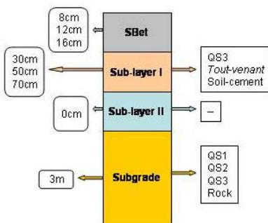
Fig. 7 – Combinations of material type and thickness for bituminous sub-ballast.
