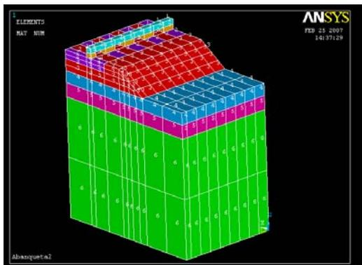
Fig. 2 – Model with ballast shoulder.
