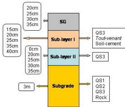
Fig. 5 – Combinations of material type and thickness for granular sub-ballast.
