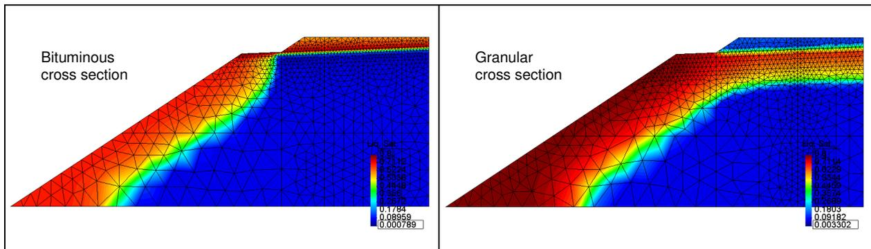
**Fig. 5 – Liquid Saturation at the end of 5 years (Original cross sections ( $\alpha = 15\%$ ))**
