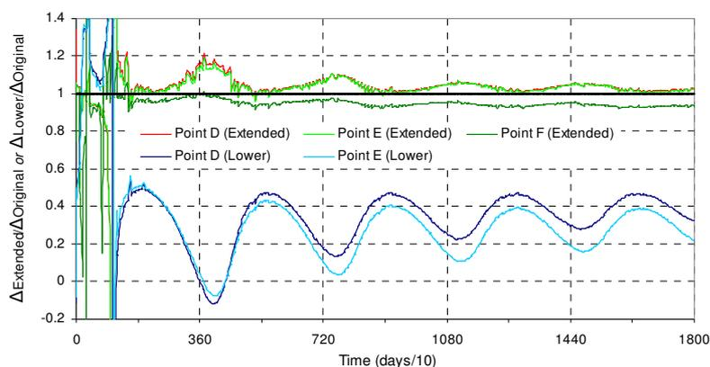
**Fig. 6 – Relation between original and alternative designs using bituminous sub-ballast**
