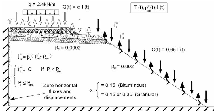
**Fig. 4 – Boundary flow rate conditions.**
