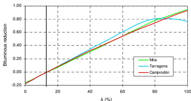
Fig. 2 – Bituminous reduction for maximum vertical displacements
