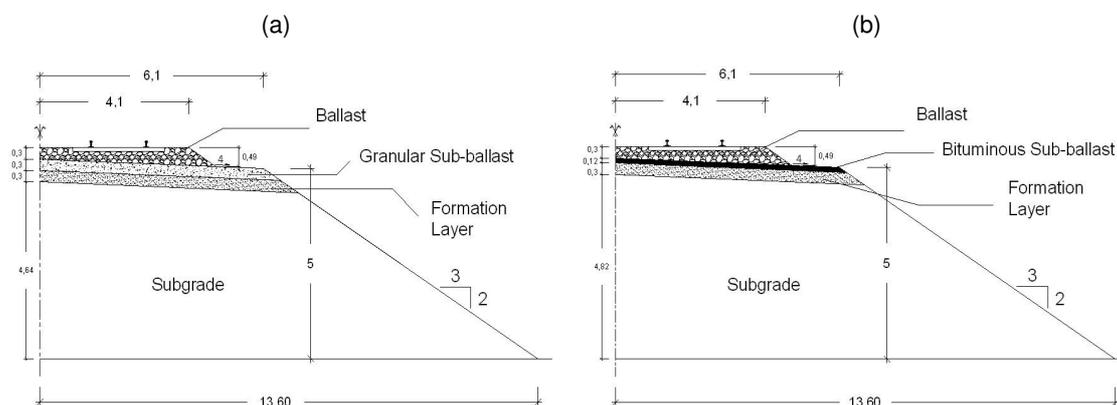
Fig. 1 – Cross sections: (a) Granular sub-ballast; (b) Bituminous sub-ballast.
