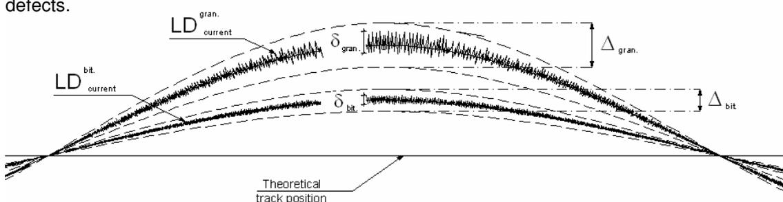
**Fig.7 – Register for Longitudinal defects: Granular vs. Bituminous**
