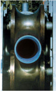
Figure 3.6 – Rolldown technique: detail on the reduction machine (Subterra, 2003)
