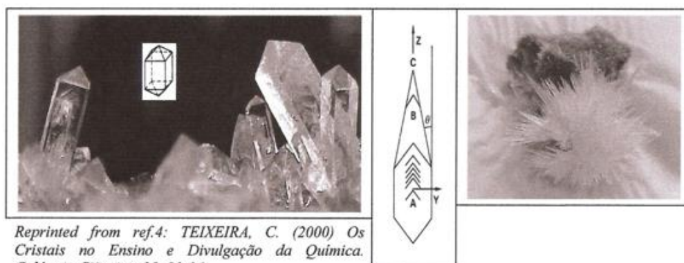
Figure 2- Left: the perfect form of pure ADP single crystals - tetragonal prism + pyramid (A). Center: scheme of the evolution for the perfect habit A, to tapered prism + pyramid B and finally, needles or whiskers C Right: acicular crystals C of ADP grown on volcanic rocks. The samples shown in both photographs are transparent.
