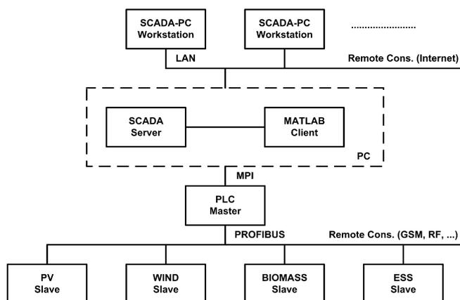
Fig. 10. Implemented communications architecture.
