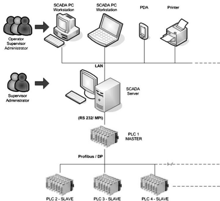
Fig. 6. PLC network and SCADA supervisory system.
