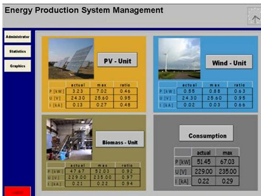
Fig. 9. Screenshot of the Energy Production System Management SCADA application.
