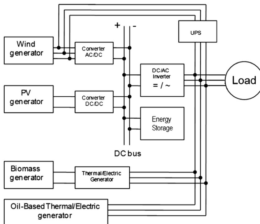
Fig. 1. Electrical structure of the PETER power supply system.
