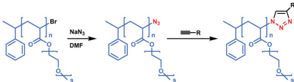
Scheme 3. General strategy for the “click” functionalization of well-defined POEGA synthesized by ATRP. 45
