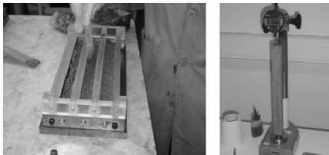
Casting of the mortar bars (left) and expansion measurement (right) in mortar bar test.
