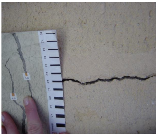
In-situ testing for renders' performance evaluation: cracks measurement (left) and adherence pull-off test (right)
