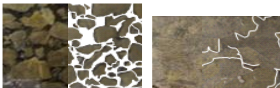
Compacted marls under 1000kPa (w=2%, s=230MPa) Compacted marls loaded full saturated until 1000kPa Oedometer tests performed under different suctions showing the physical degradation of the fragments
