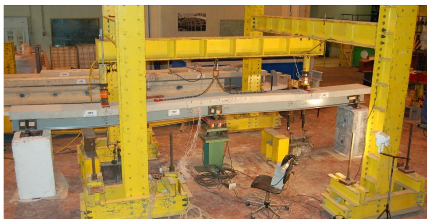
Flexural test on a 2-span GFRP-concrete hybrid beam.
