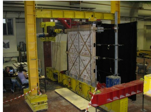
Cyclic test of an ordinary timber-masonry wall
