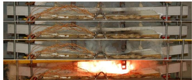
Fire resistance tests on GFRP beams protected with calcium silicate: failure sequence (time interval, approximately 1 s.)
