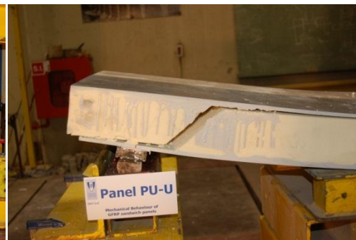
Flexural tests on sandwich panel: shear failure in polyurethane core.
