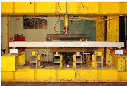
Flexural tests on sandwich panel: test setup.
