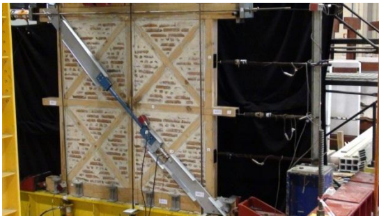
Cyclic test of a timber-masonry wall with an elastic-plastic dissipative device
