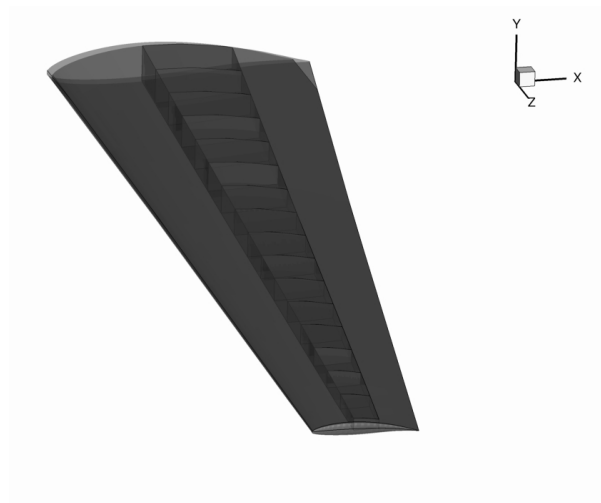
(f) Aero-structural combination for the L-23 wing geometry.
