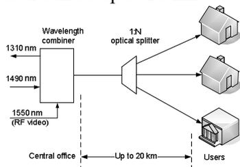
**Figure 2.2. Typical GPON architecture**
