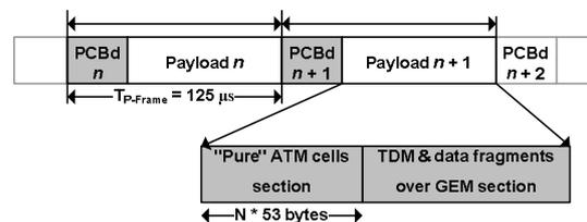
Figure 4.1. Downstream GPON frame
