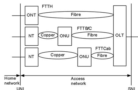
**Figure 2.1. FTTx network architecture**
