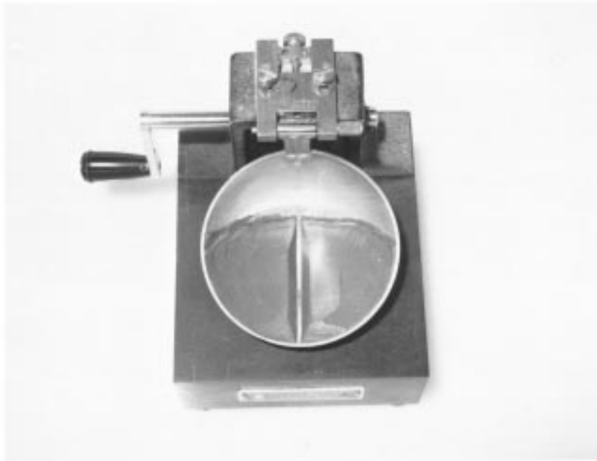
FIG. 6 Grooved Soil Pat in Liquid Limit Device
