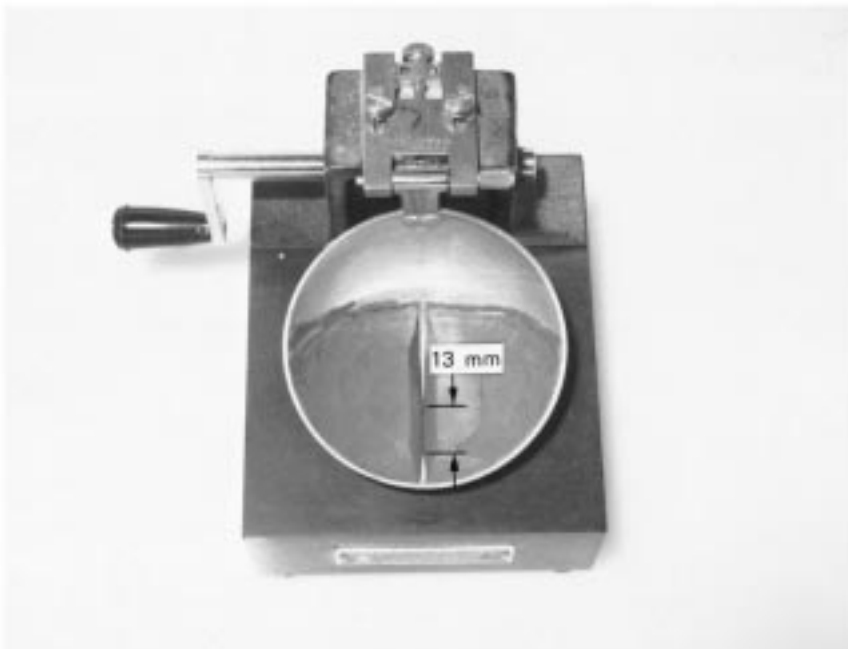
FIG. 7 Soil Pat After Groove Has Closed
