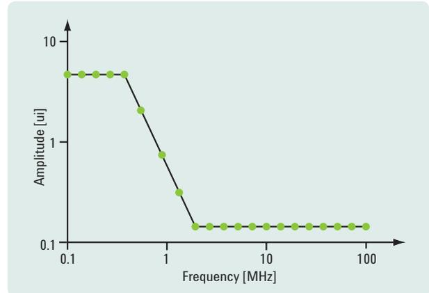
**Figure 3. Compliance test with a sinusoidal jitter tolerance mask. Green dots show measured points that passed a BER test at  $10^{-12}$ .**
