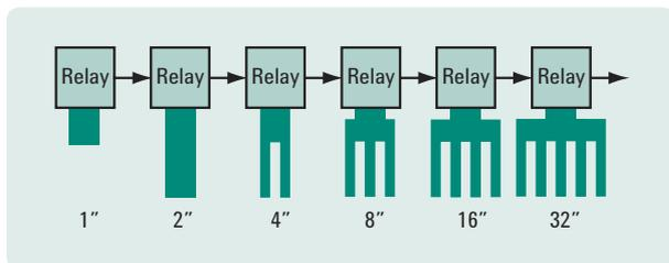
**Figure 8. ISI generation using a backplane with switchable traces**
