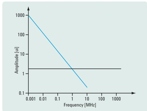
Figure 6. Maximum sinusoidal jitter amplitude, as a function of jitter frequency. Blue line: frequency/phase modulation; Black line: delay modulation.
