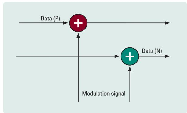
**Figure 9. Level interference circuit using passive adders**
