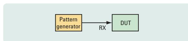
Figure 1. High-level setup for a receiver tolerance test
