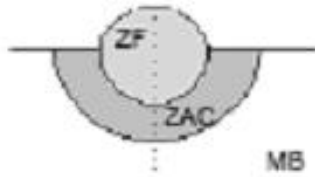
Figure 3 - Illustration of the hardness measurements.
