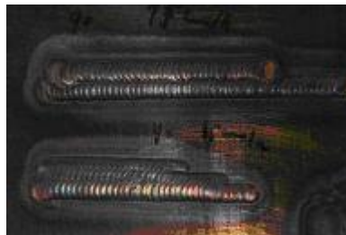
Figure 2 – Illustration of Multipass welding
