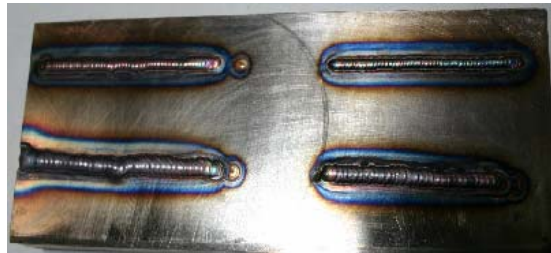
Figure 4 - TIG weld deposits.
