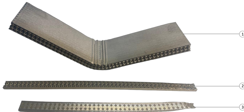
Figure 3.16: EDM post-processing fragments (1) RTCO-025-02-2 samples (2) rows of cells that were excessively cut (3) support used while printing the sample.
