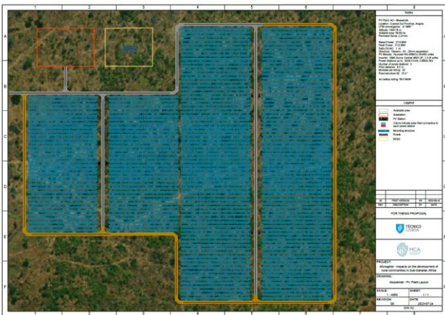
Figure 7 - Mussende PV Park Layout (Source: PVCase)
