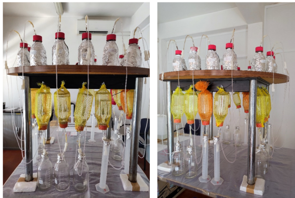
Figure 1: Experimental setup - reactor bottles (on the top of the table), inverted bottle filled with NaOH solution (packed in colorful nylon nets), measuring cylinders or empty bottles as recovery system.
