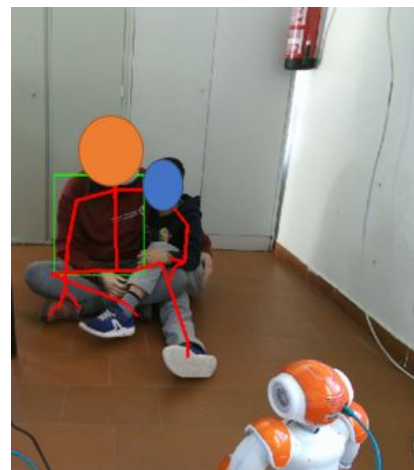
Fig. 1. Example of challenging position during therapy captured by the Kinect camera. The represented skeleton is a hybrid of the upper body of the therapist and the lower body of the child (extracted from [4]).
