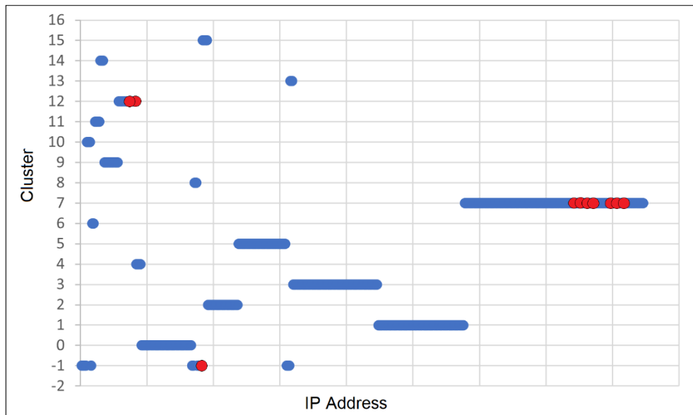
Figure 5 - Machine distribution by cluster with DSCAN algorithm for x=20 and host data on 02-03-18, with the victims represented in red.
