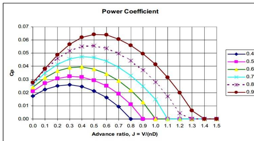
Figure 4.4: Power coefficient versus advance ratio, p/D a parameter [31]
