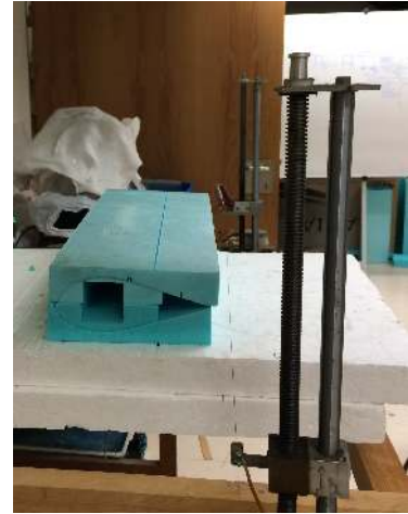
(b) Airfoil already cut and ready to be covered
