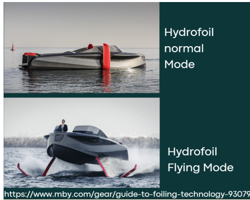
Figure 1: Two different modes of a hydrofoil. The normal mode is characterized by low-speed/high-drag while the flying is high-speed/low-drag.
