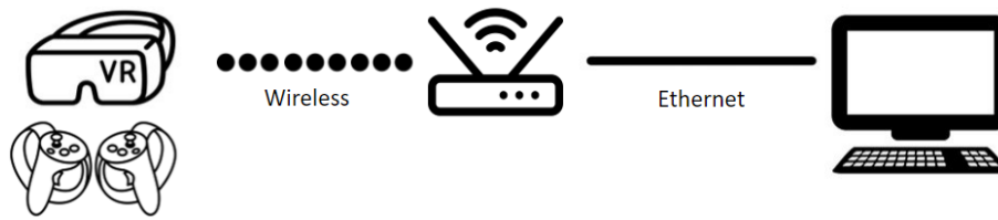
Figure 5.11: Diagram of the test apparatus used for the second user test, featuring improvements based on feedback from the pilot of this user study. In contrast to the cable used in the first user test, a LAN connection was implemented.
