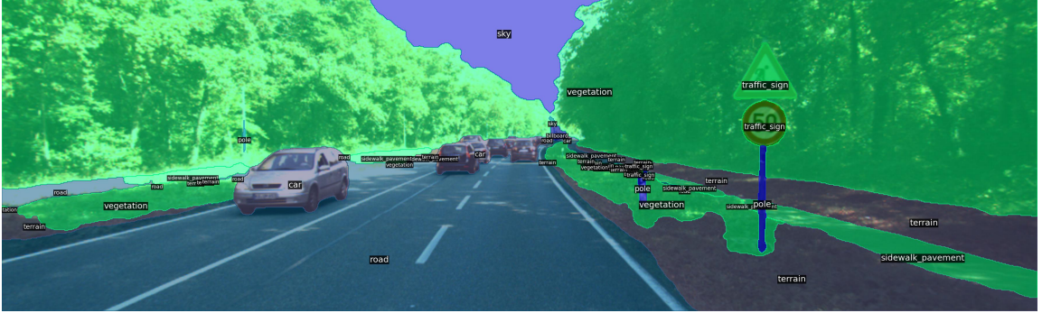
Figure 4.5: Semantic segmentation labels overlaid on the RGB image from Fig. 4.4
