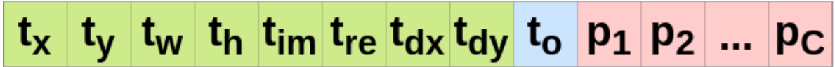
Figure 4.11: A bounding box predicted by the 3D Object Detector and Tracking module. Two extra parameters are learned in order to predict a bounding box's displacement between two consecutive frames, t_{dx} and t_{dy} .
