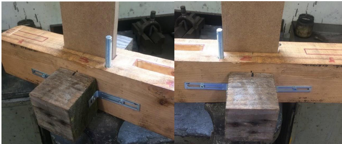
Figure 3.4: Close-up of the fixed vertical support ( encastre ), stabilized by two blocks. This platform block then rotated around the axis of a 20 cm steel screw
