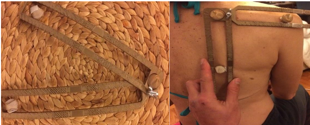
Figure 3.3: (a) Final assembly of the two 3-D printed parts and (b) scapula locator in use, locking the subject specific scapula configuration
