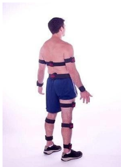
Figure 3.6: FAB system from Biosyn, Canada. This inertial measurement units setup was used, with the exception of the sensors in the lower limbs
