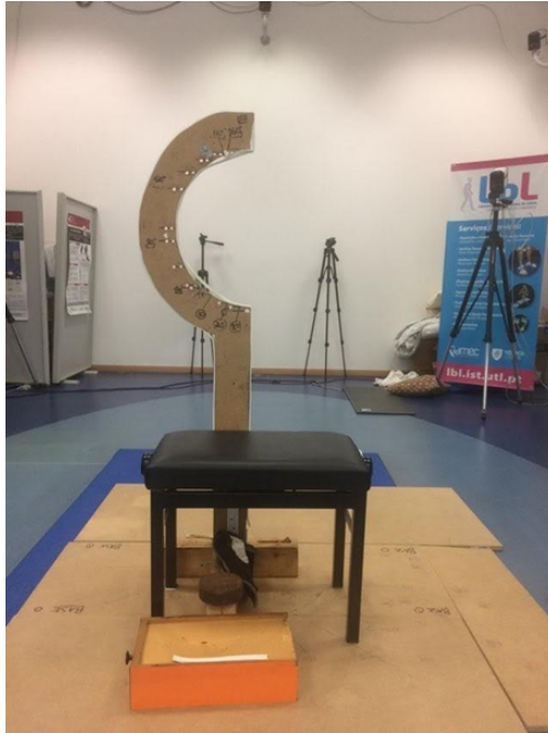
Figure 3.5: Overview of the built external frame, which rotated around the axis of a 20 cm steel screw, fixed ( encastre ) in the panel laid on the laboratory's floor, where marks had been drawn signalling the different elevation planes. In front of the frame the height adjustable bench and the support for the participant's feet, which aimed at minimizing thorax flexion, are displayed
