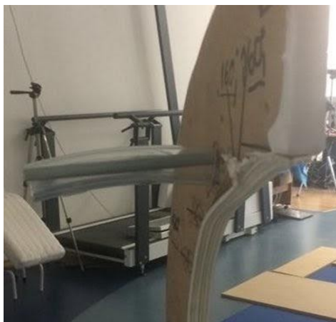
Figure 3.8: Close up of the platform where the participant laid his arm, at the selected elevation angle. The latex cover reduced skin abrasion
