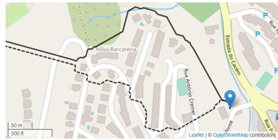
Fig. 10: Closeup of the final part of the path from IST Tagus to Location1, distance between way-points from 2 with margin to buildings of 10 meters with dynamic updates (dashed path) and static updates (solid path) to the graph edges.
