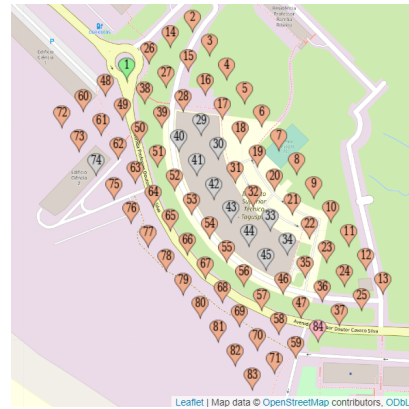
Fig. 2: Pinpoints’ of a small resolution grid for obstacle detection, with start point on #43 (green), goal point on #56 (purple), and the detected points in grey.
